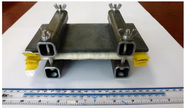
**Fig.3. Fabrication of supercapacitor stack with 6 cells, each cell 18x27 cm<sup>2</sup>**
