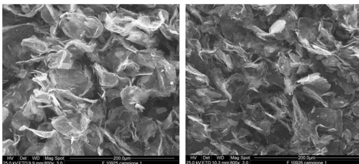
The softness of the single nanoplatelets can be explained assuming that each layer is made of very few graphene layers.
