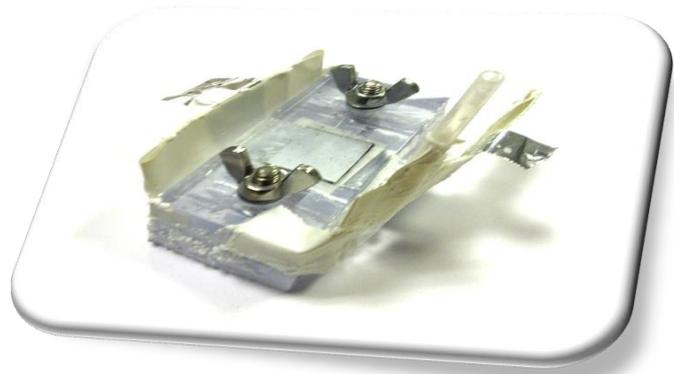
**Fig.2. Small supercapacitor cells (a) after fabrication and (b) in the test frame**
